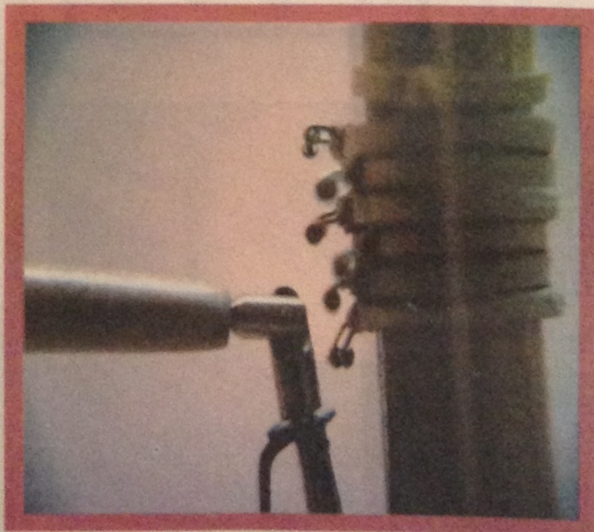
The hoops holding a catboat's sail were painstakingly made from layers of wood shavings, glued like plywood.
